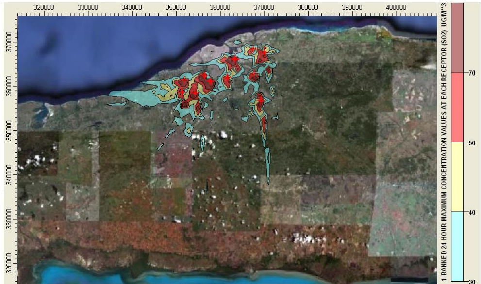
Fig. 6. Isolines of the maximum hourly concentration of SO 2 . (Source: Base Map Google Earth)
